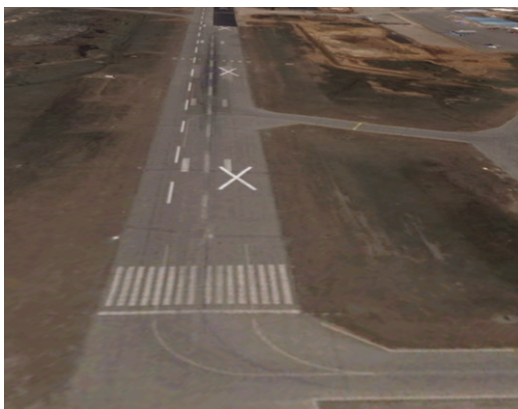
Aerial view of the runway markings used at the Iqaluit Airport during construction
