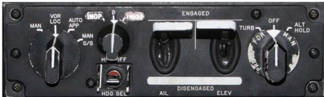
Photo 7. Autopilot mode control panel (AP MCP)
