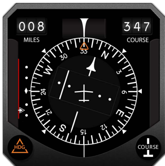
Figure 16. 1639:10: Captain's horizontal situation indicator (HSI), indicating 17° intercept angle (no. 2 compass with -16° heading error)
