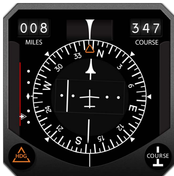
Figure 17. Exemplar of captain's HSI (no. 2 compass) indications at 1639:10, had there been no heading error
