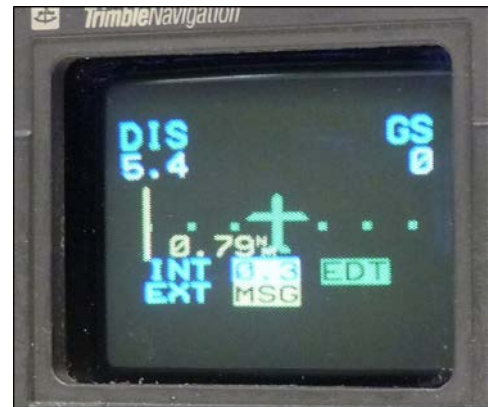
Photo 2. TNL-8100 control display unit (CDU) screen, showing right-of-track indication
