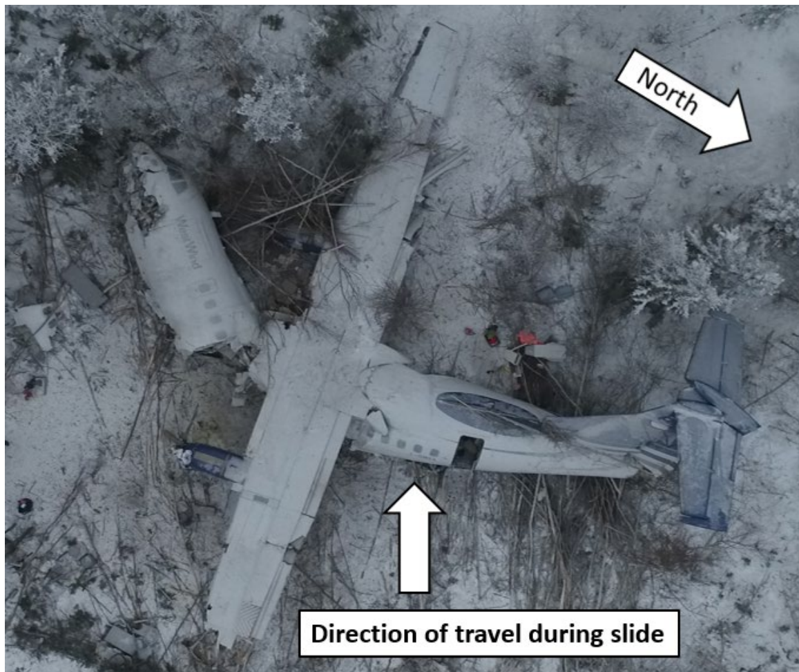
Figure 9. Photo of aircraft wreckage, as seen from above (Source: Royal Canadian Mounted Police, with TSB annotations)
