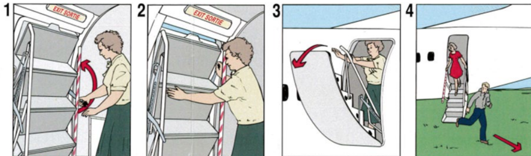
Figure 27. In-flight safety card pictorial instruction of how to open the main exit door (Source: West Wind Aviation L.P.)
