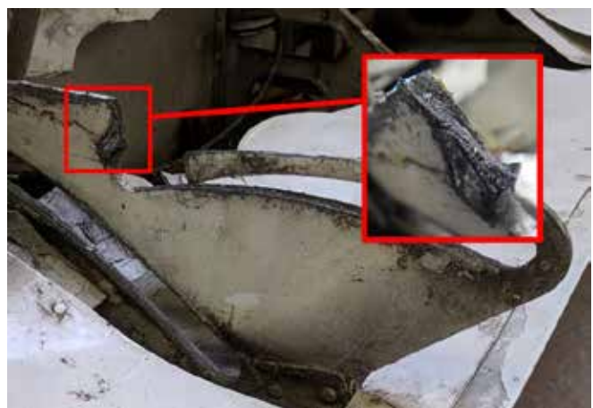
Figure 1. The fractured flap track, with an expanded view of the fractured area
