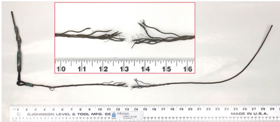
Figure 1. Fractured nose-up elevator control cable
