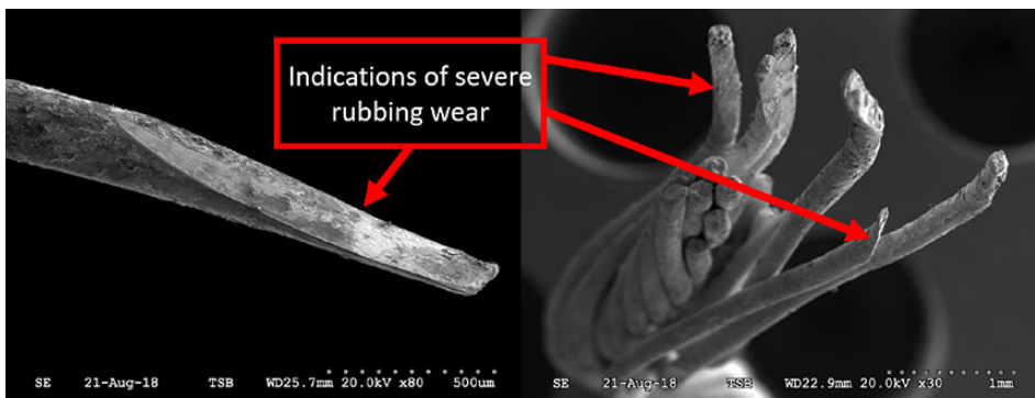
Figure 2. Micrograph of the nose-up elevator control cable's fractured surfaces
