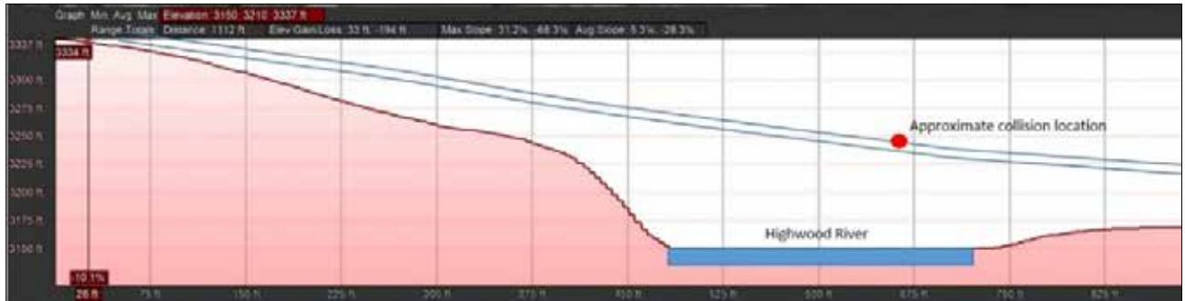
Figure 4. Profile of terrain and location of power transmission line relative to the Highwood River, looking east toward the direction the helicopter was coming from (Source: Google Earth, with TSB annotations)
