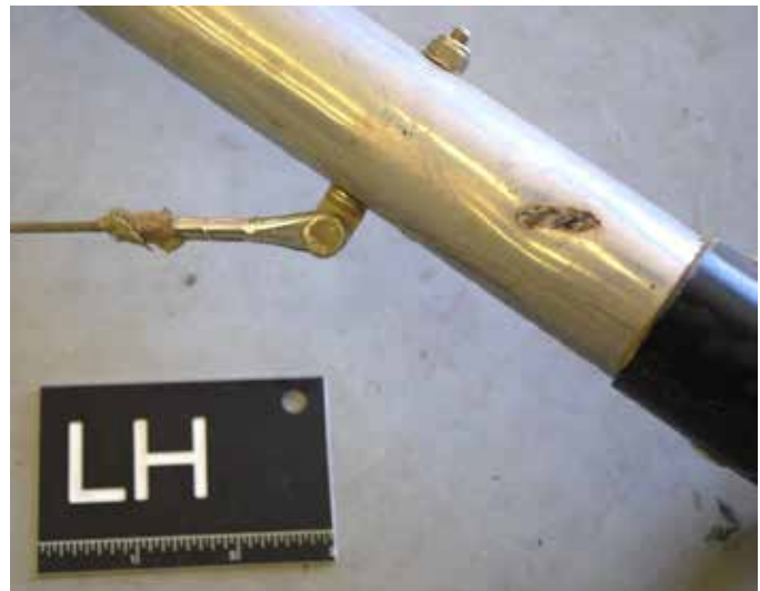
Figure 3. Close-up of lower left-hand cross-tube wire-strike mark
