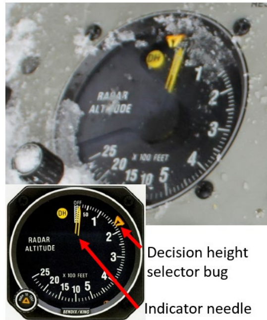
Figure 2. Radio altimeter on the occurrence aircraft (Sources: TSB [main image] and manufacturer's brochure [inset image])
