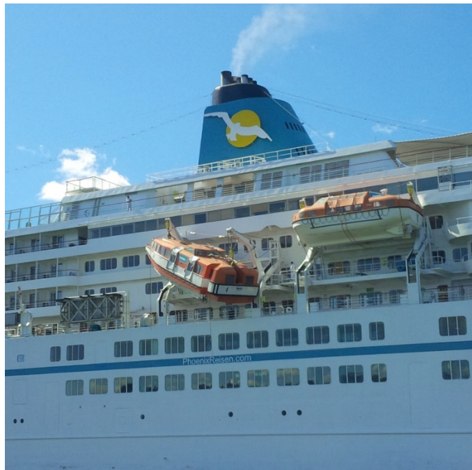
Figure 10. Lifeboat No. 4 following the uncontrolled lowering of the davit's aft arm (Source: TSB)
