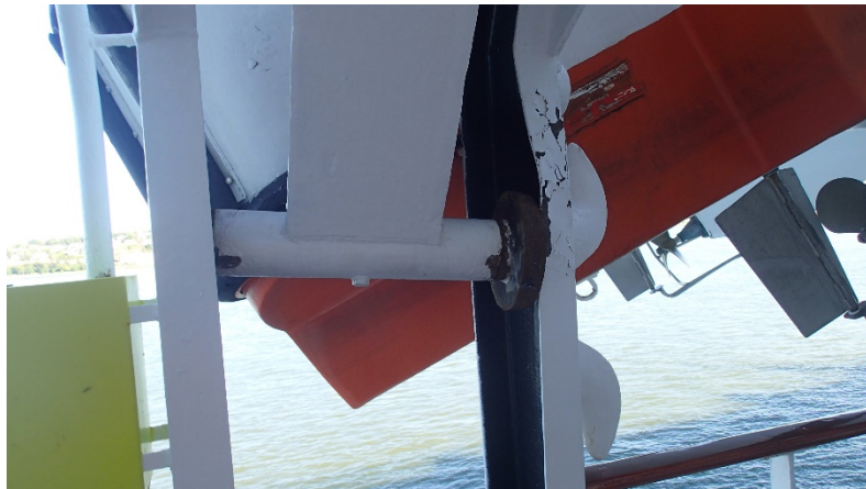
Figure 11. Damage sustained to lifeboat No. 4 davit aft roller track (Source: TSB)
