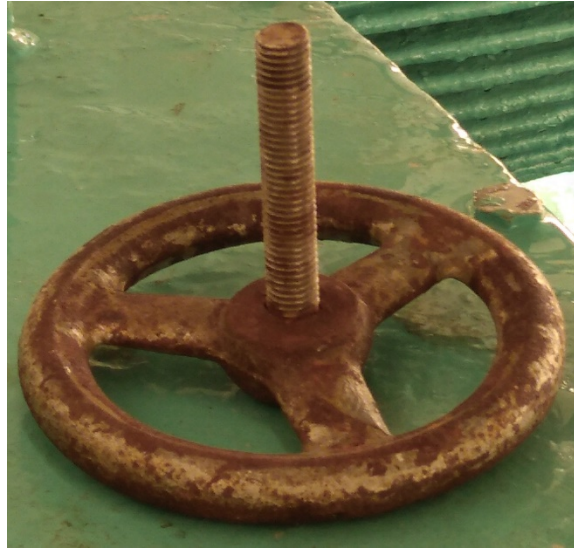
Figure 3. Brake release tool for the winch motor's electromagnetic brake (Source: TSB)
