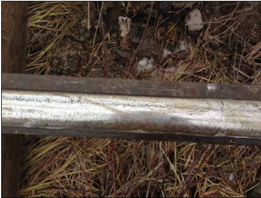
Photo 2. Wheel flange marks on the head of the low rail
