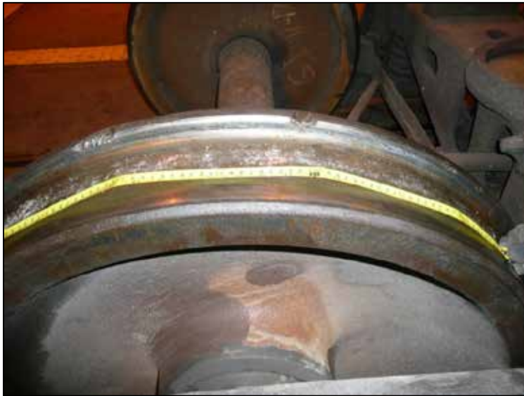
Photo 3. Impact marks on L-4 wheel flange and tread
