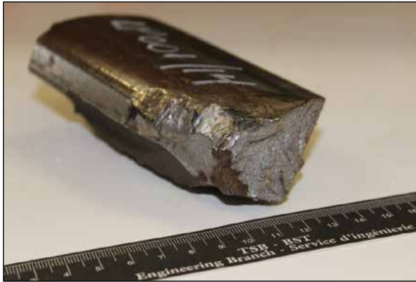
Photo 6. Piece of high rail showing batter and wheel strike marks
