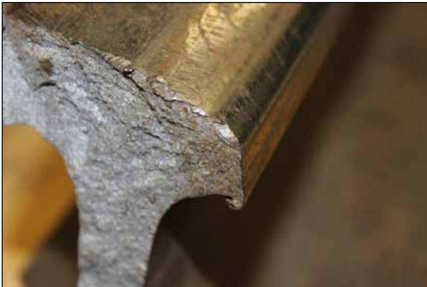
Photo 5. Small detail fracture on gauge corner
