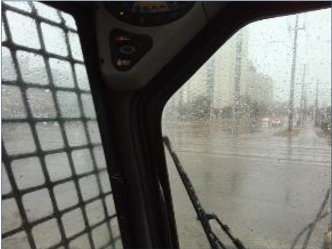
Figure 5. Photo taken from a driver's seated eye position in the snowplow showing the view toward the northwest quadrant of the crossing when the snowplow was positioned adjacent to the southeast quadrant crossing warning system mast (the location of the snowplow when the gates began to descend) (Source: TSB)
