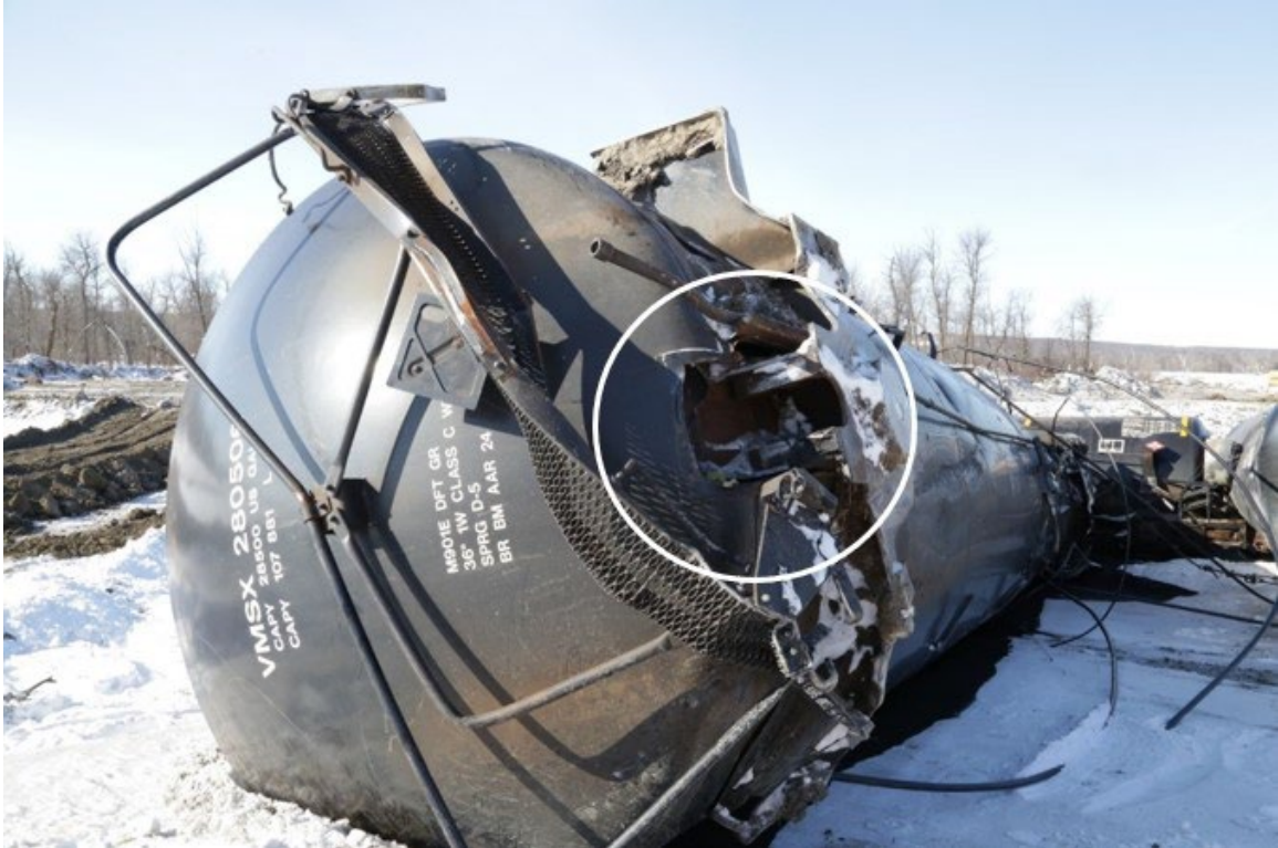
Figure 18. Tank car VMSX 280506 stub sill separation (Source: TSB)
