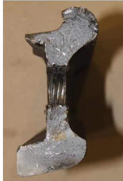
Figure 15. Imprints of bolt threads were worn into a gauge-side 132/136 RE compromise joint bar bolt hole of rail end B
