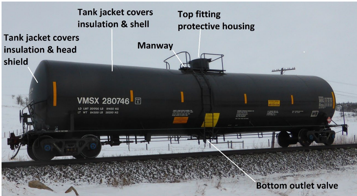
Figure 16. General arrangement of Class 117R tank car VMSX 280746 (5th car from head end) after being re-railed. A tank car jacket and insulation encase the tank shell and full head shields. The pressure relief devices are located inside the top fitting protective housing. (Source: TSB)
