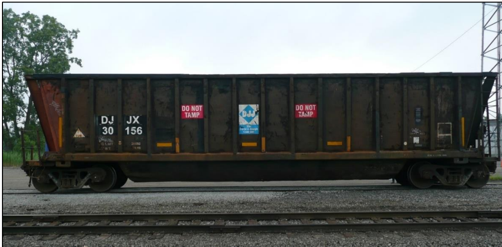
Figure 22. Side view of DJJX 30156 (line 13) bathtub gondola car, which was a car of the same design as DJJX 30478 (Source: TSB)
