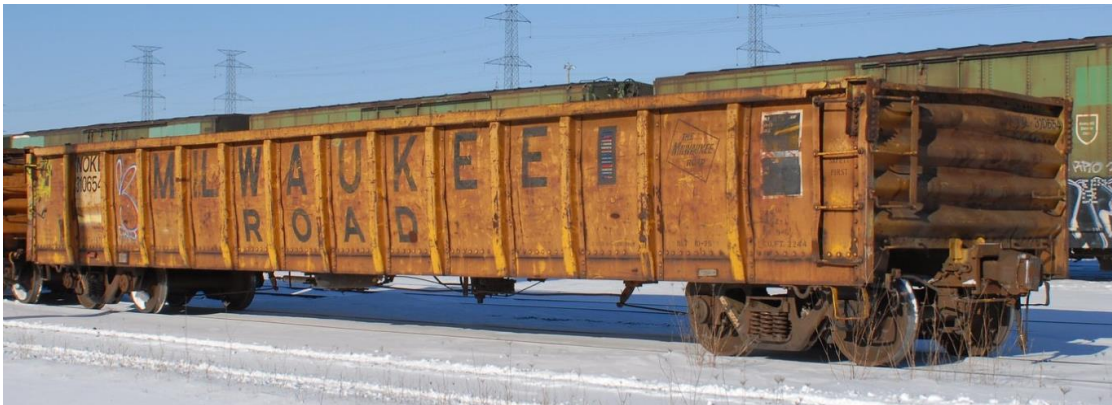
Figure 21. Typical flat-bottomed gondola car (Source: I. McCord)
