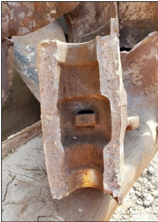
Figure 7. Fracture surface of the broken A-end knuckle on car DJJX 30478 (line 53) (Source: TSB)
