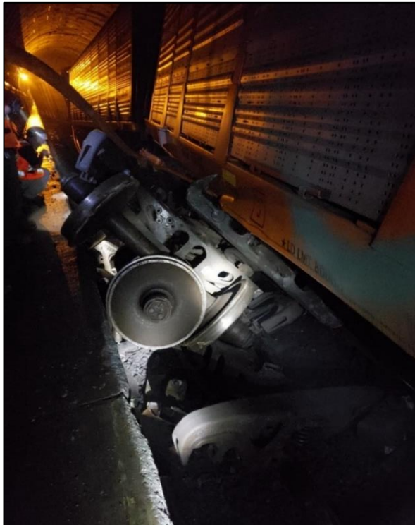
Figure 13. Displaced wheel sets, trucks, and derailed cars on the Canadian side (Source: TSB)
