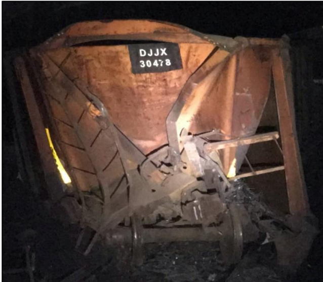
Figure 30. DJJX 30478 AL failure in tunnel (Source: Federal Railroad Administration)
