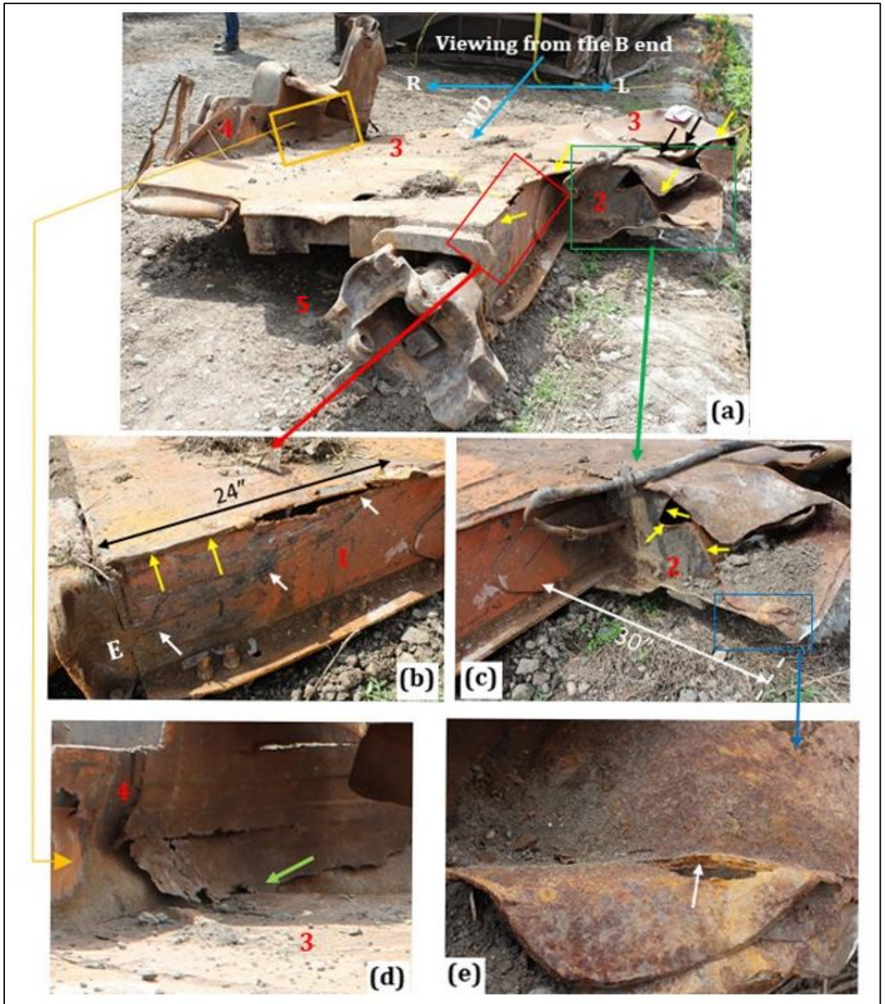
Figure 27. Car DJJX 30478 A-end wreckage in upright position. Photo (a) is an overview; photos (b), (c), and (d) are the close-up views of the red, green, and yellow boxes in (a), respectively; photo (e) is a close-up view of the blue box in (c). (Source: TSB)
