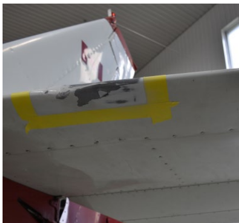
Figure 3. Damage to C-GRAE's horizontal stabilizer (Source: TSB)
