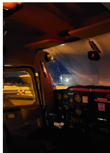
Figure 5. Inside C-GRAE's cockpit at night, with lighting from the red ceiling light (Source: TSB)
