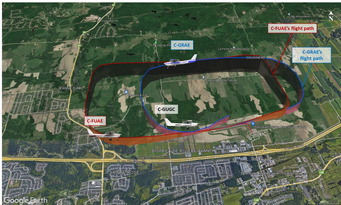
Figure 1. Map showing the positions of the 3 aircraft in the circuit in preparation for the 2nd touch-and-go (Source: Google Earth, with TSB annotations)
