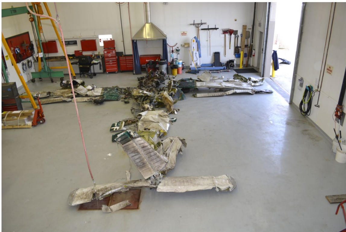
Figure 4. Layout of aircraft wreckage at the TSB regional office in Edmonton, Alberta (Source: TSB)
