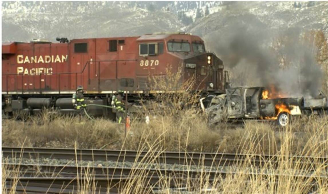
Figure 3. Destroyed hi-rail vehicle after the collision (Source: CFJC Today)
