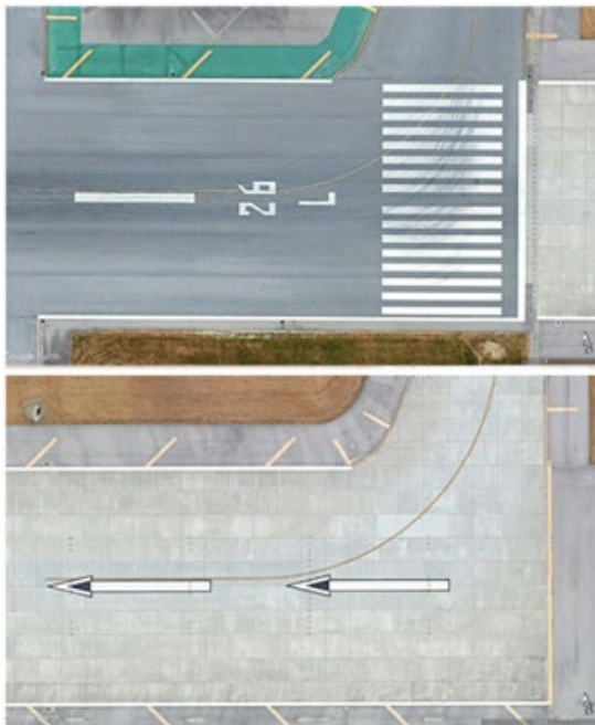
Figure 6. Runway threshold (top) and displaced threshold area (bottom) at Vancouver International Airport (Source: Google Earth)
