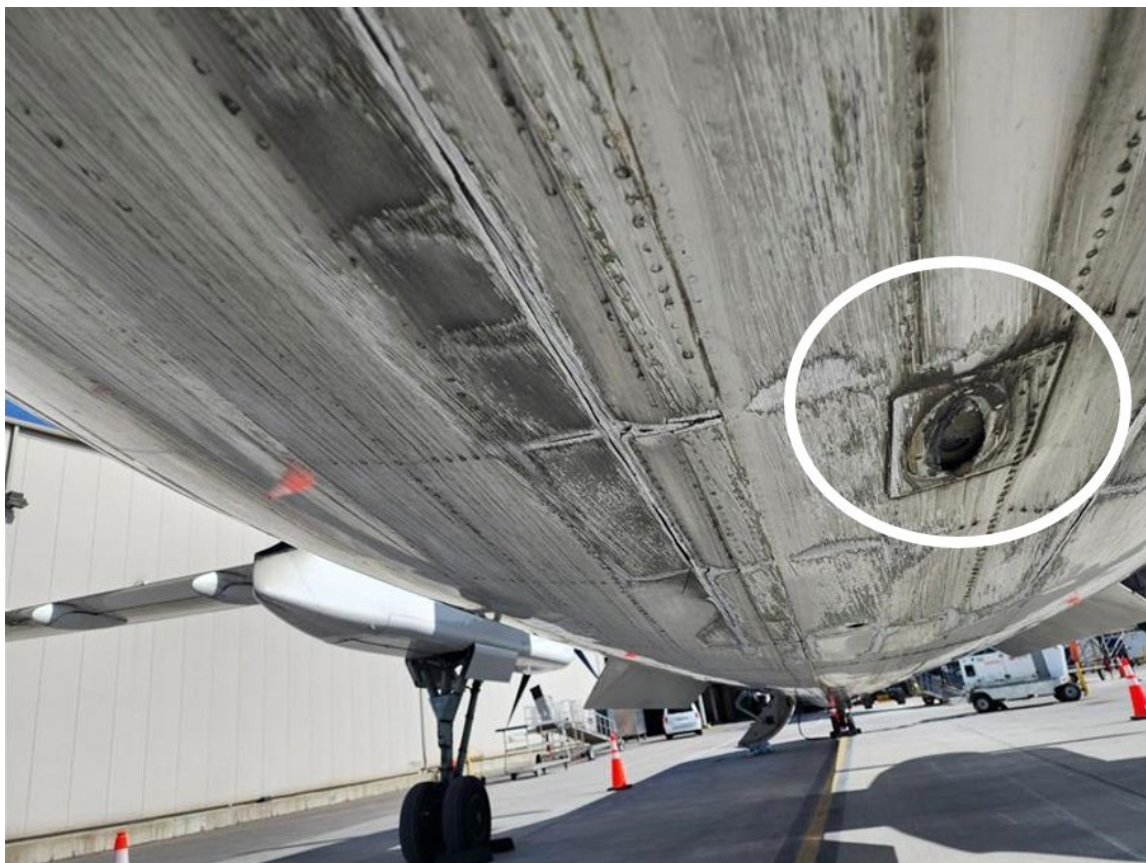
Figure 1. Lower aft fuselage damage and broken off tail strike switch on the occurrence aircraft (Source: Third party [with permission], with TSB annotations)
