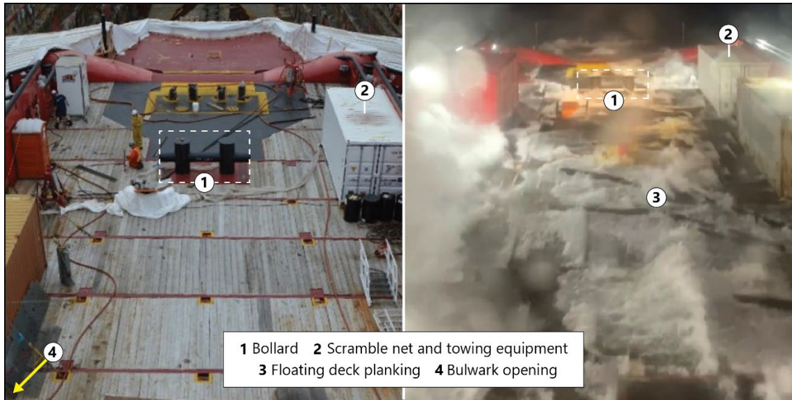
Figure 3. Photos of the aft deck of the Jean Goodwill while in dry dock (left) and during the occurrence (right), showing the bollard in the centre and the containers for the SAR equipment and the towing equipment (Source of left image: TSB. Source of right image: Canadian Coast Guard crew member)
