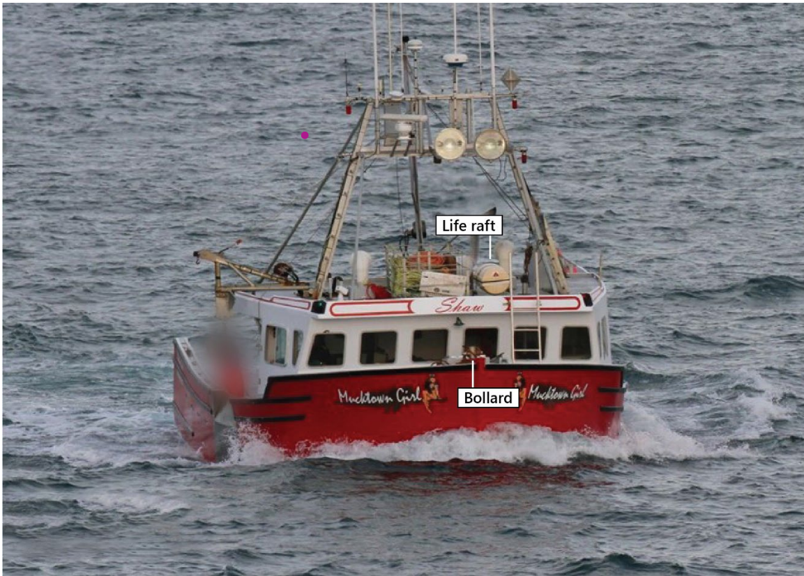
Figure 1. The fishing vessel Mucktown Girl , showing the bollard that the towline was attached to and the location of the life raft (Source: Steven Kennedy)
