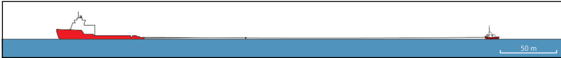
Figure 6. Diagram of the towing arrangement showing the relative sizes of the Jean Goodwill and the Mucktown Girl and the length of the towline (Source: TSB)
