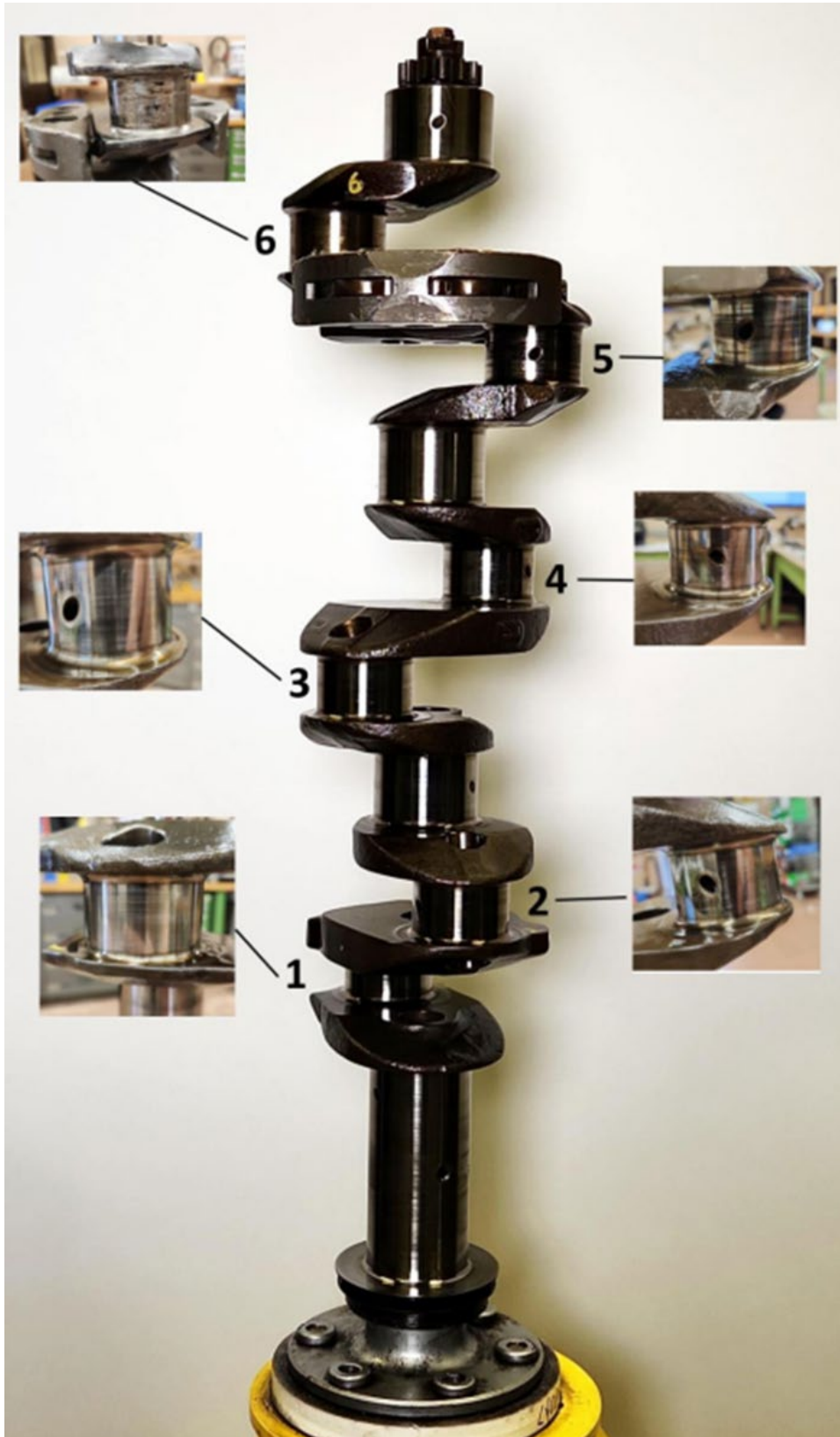
Figure 3. Scoring marks on the crankshaft rod bearings (Source: TSB)
