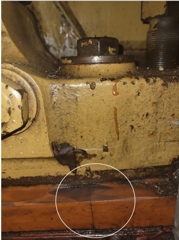
Figure 9. Close-up photo of engine mounting, showing a crack on the forward port engine mount near the bolts (Source: TSB)
