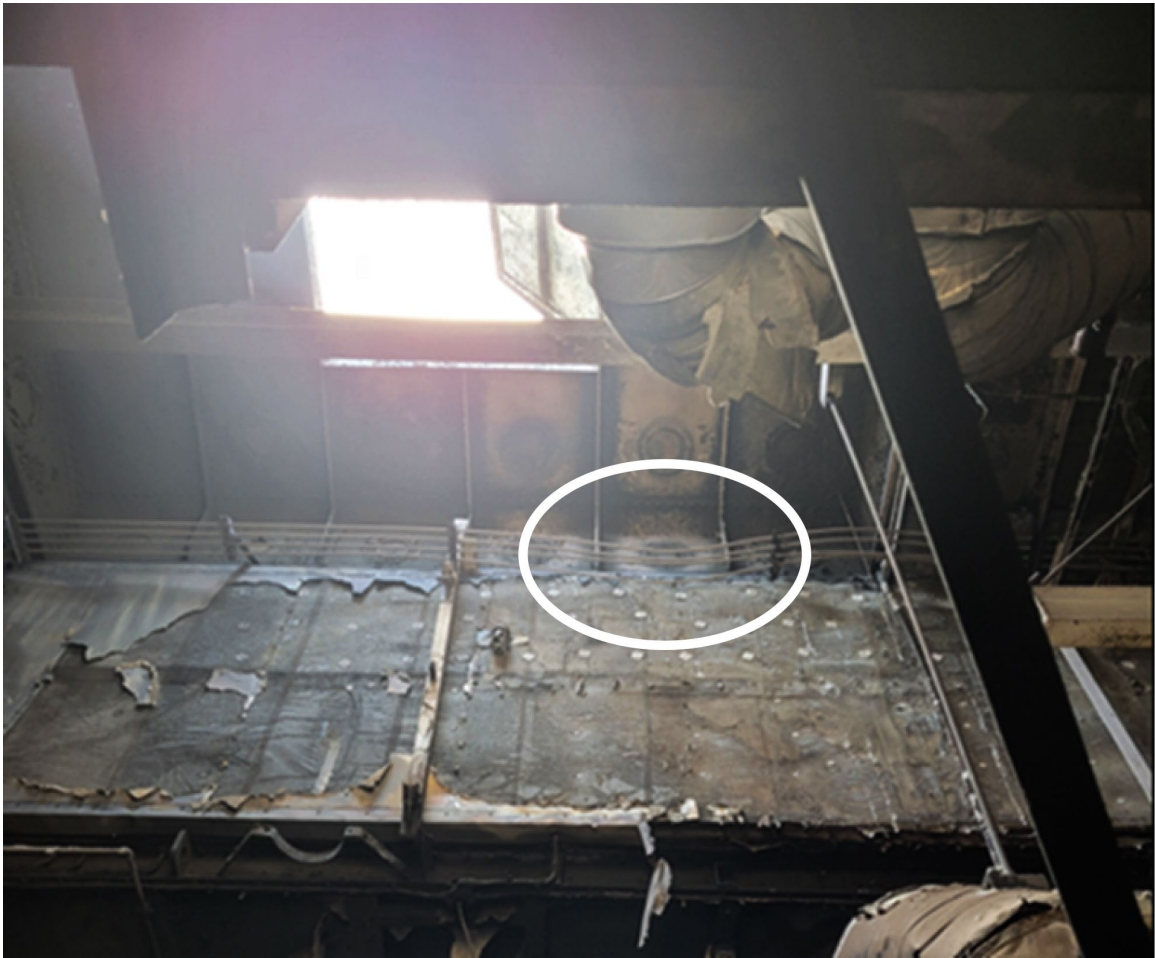
Figure 17. The conduits for the remote release cables passed close to the skylight and the cables were damaged in the fire (circled location). The insulation on the boundary between the engine room and accommodation spaces was partially destroyed. (Source: TSB)
