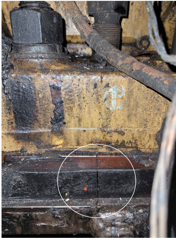
Figure 11. Close-up photo of engine mounting, showing a crack on the aft port engine mount near the bolts (Source: TSB)
