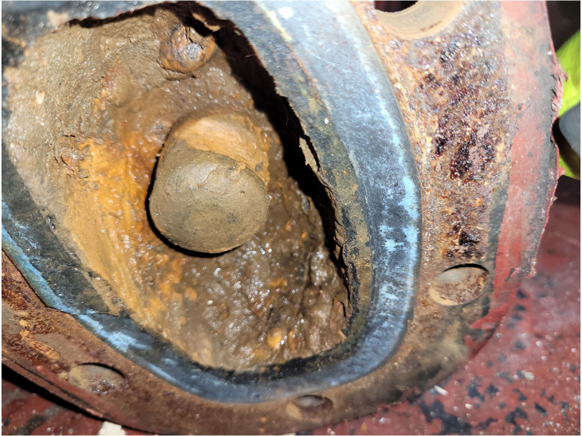
Figure 20. The isolation valve disassembled, showing the disconnected spindle (Source: TSB)
