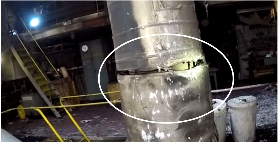
Figure 12. Insulation on turbocharger showing gaps in the way the insulation had been installed on the turbocharger outlet from the side (Source: TSB)
