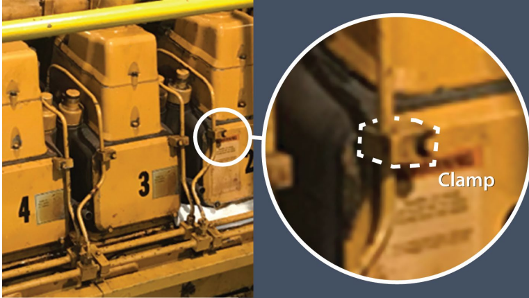
Figure 7. Main engine after the occurrence showing fuel injection lines with only bolts at the location for the retaining clamps (1 enlarged) (Source: TSB)
