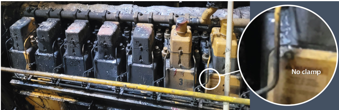
Figure 7. Main engine after the occurrence showing fuel injection lines with only bolts at the location for the retaining clamps (1 enlarged) (Source: TSB)
