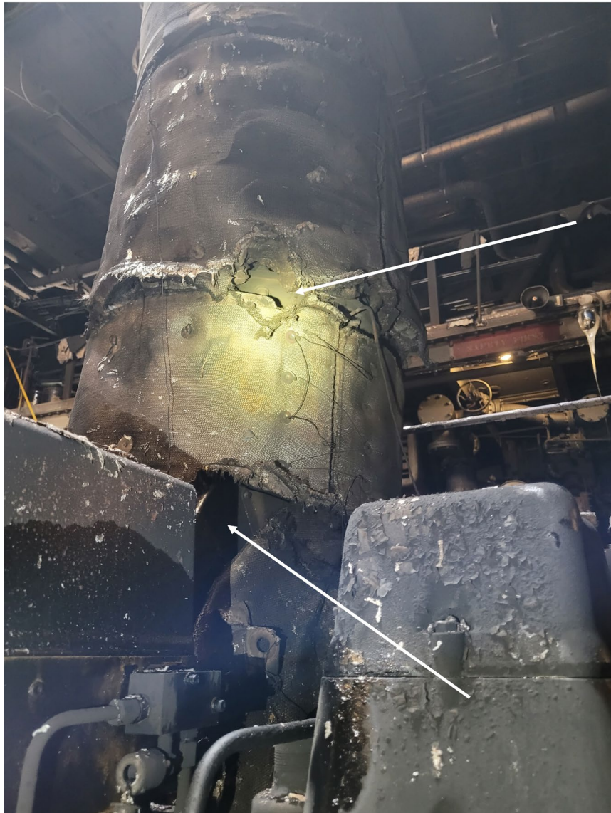
Figure 13. Insulation on turbocharger showing a notch in the way the insulation had been installed on the turbocharger outlet (Source: TSB)
