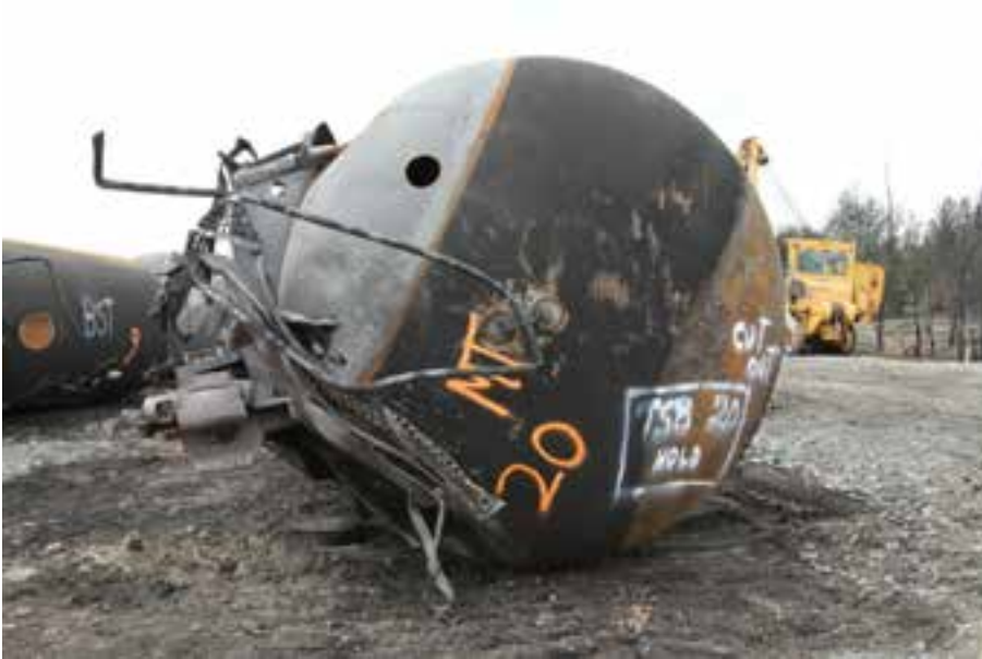
(a) Coupon marked on the head.
