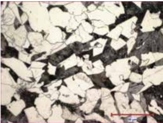
(d) Optical micrograph taken in the middle of the cross-section (Nital etch, original magnification 200X).
