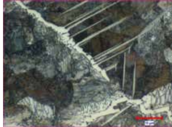
(c) Optical micrograph taken near the inner surface (Nital etch, original magnification 1000X).
