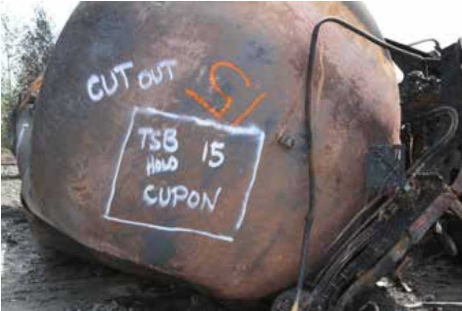
(a) Coupon marked on the head.
