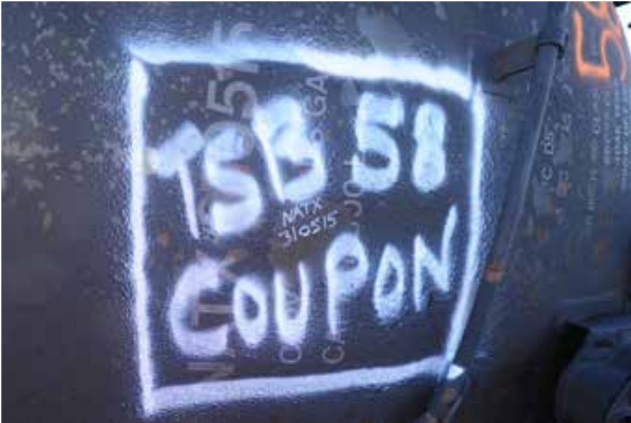
(a) Coupon marked on the head.
