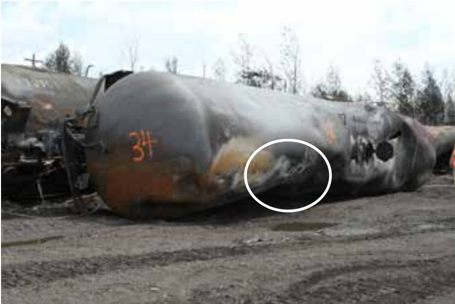
Figure 6: Photograph showing the location (circled) from which a coupon was taken from tank car WFIX 130571.
