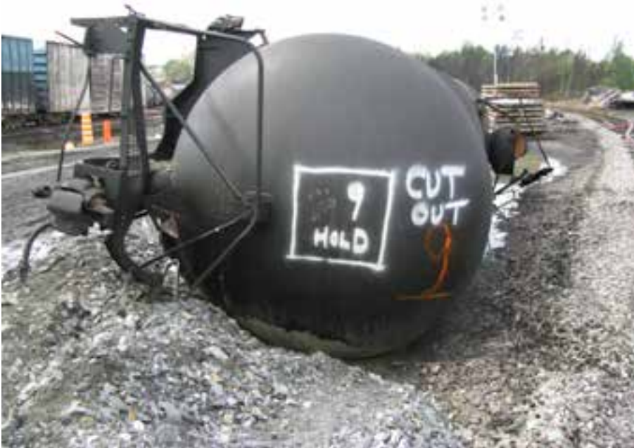
(a) Coupon marked on the head.
