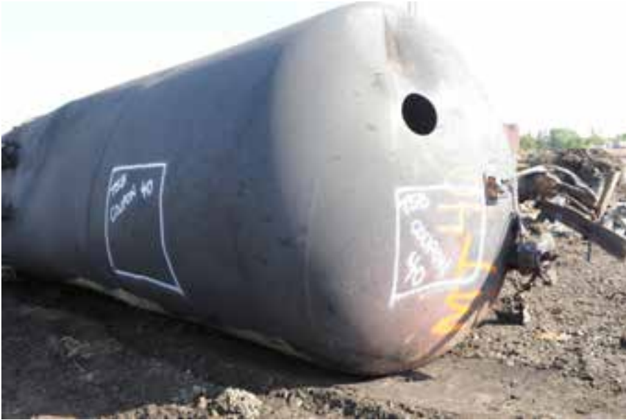
Figure 7: Photograph showing coupons marked the head and shell of tank car CTCX 735572.
