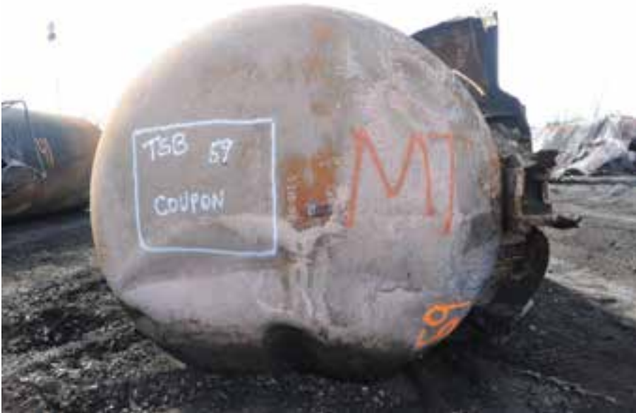
(a) Coupon marked on the head.
