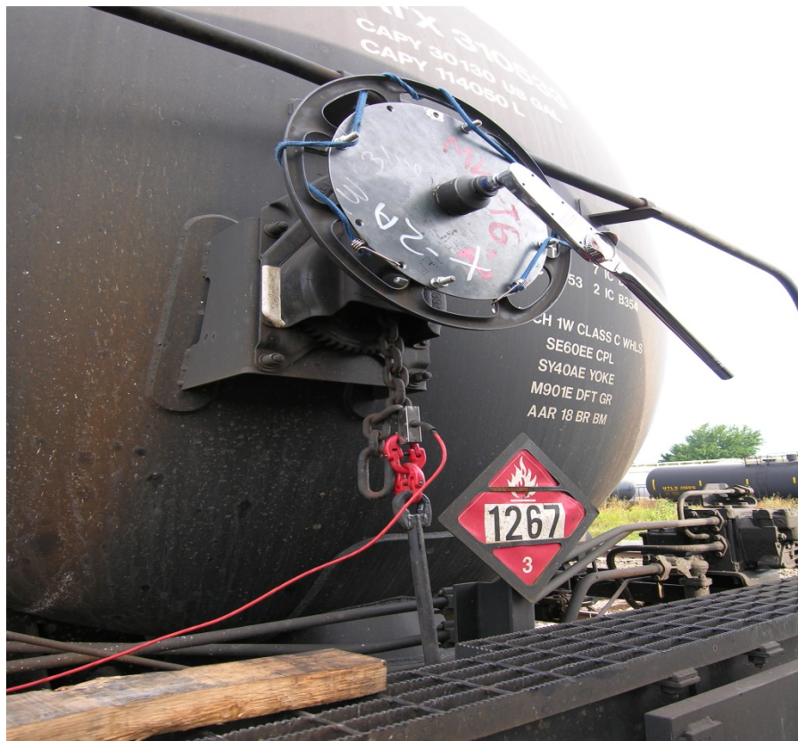
Figure 10: Inserted Chain Force Sensor and Torque Ranger
