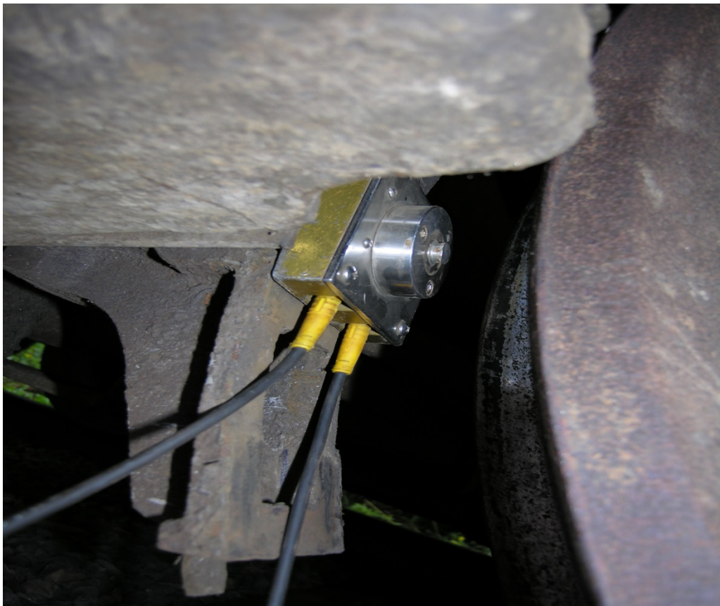
Figure 8: Jim (Golden) Shoe Sensor
