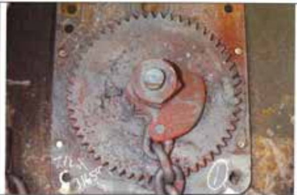
Fig 6. Ring gear of handbrake 1 Note uniform gear tooth pitch
