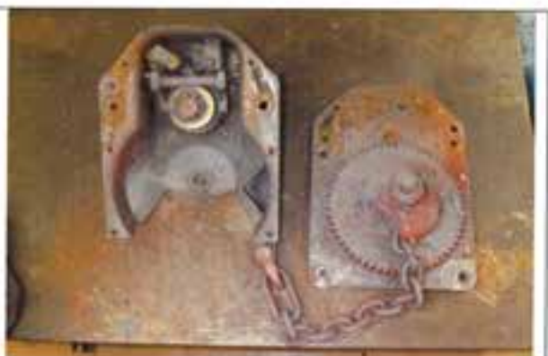
Fig 4. Handbrake 1 showing housing removed
