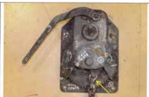
Fig. 2. Handbrake 2 handwheel removed Note white paint residue on chain (arrow)
