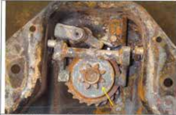
Fig 5. Pinion gear of handbrake 3 Note uniform gear tooth pitch (arrow)
