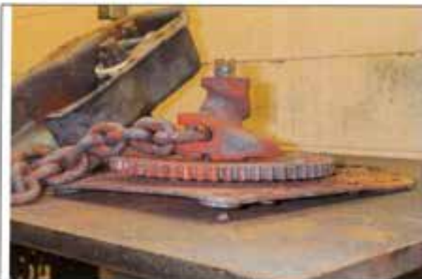
Fig 3. Handbrake 1 showing back plate deformation
