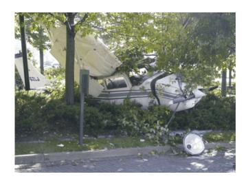
While on approach to the clearing, it appeared to the pilot that the ground was on a downslope. During the pilot's flight training, it was shown that landing on soft ground with a downslope may result in the landing gear digging in and the aircraft flipping over. Aware of this possibility, the pilot chose to stall the aircraft into the trees to reduce impact forces and injuries.
