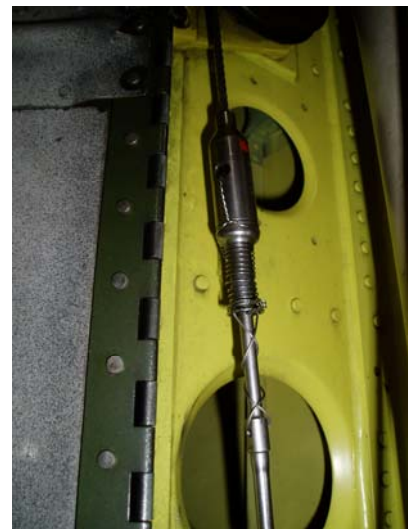
Photo 2. Properly lock-wired speed rig
