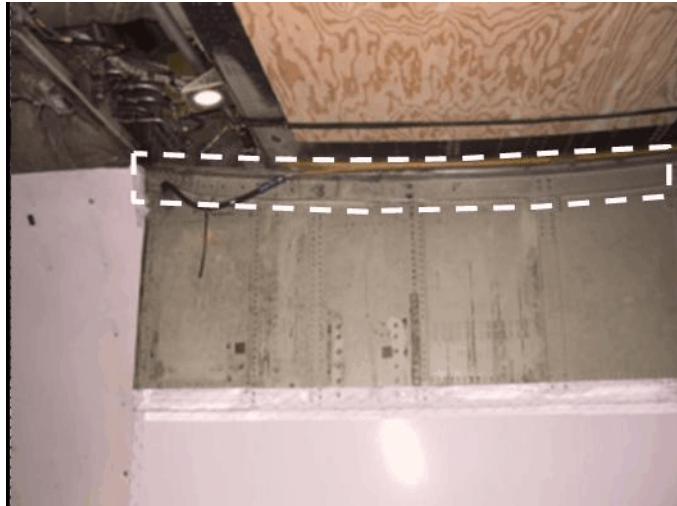
Photo 1. Dashed lines indicate wing attach angle.
