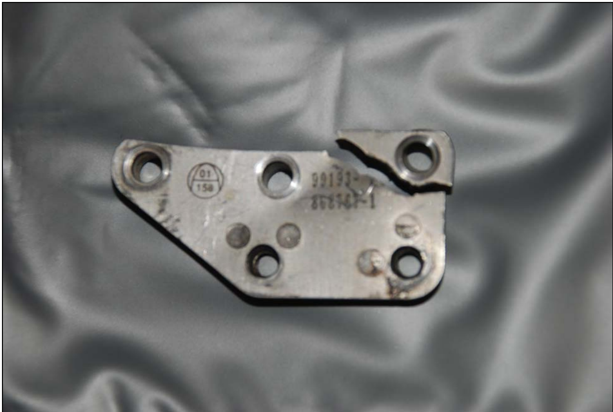
Photo 1. Left engine fuel control upper support assembly
