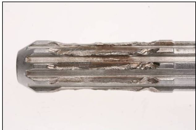
Photo 5. Close-up of external spline wear
