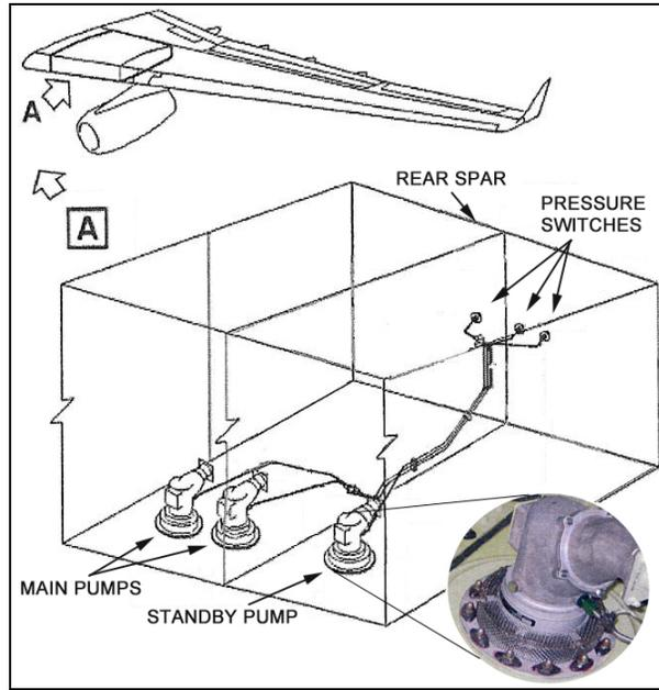
Figure 2. Fuel pumps and pressure switches
