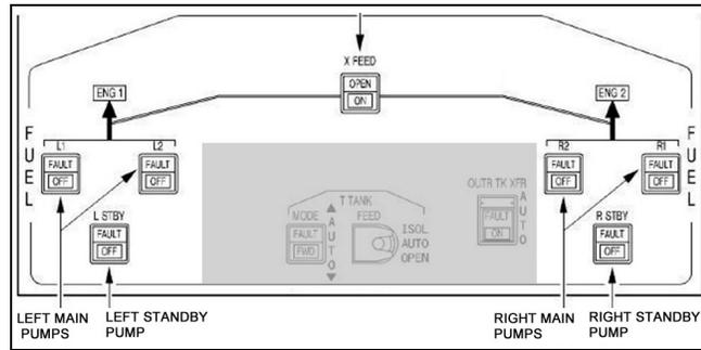
Figure 4. Fuel system controls
