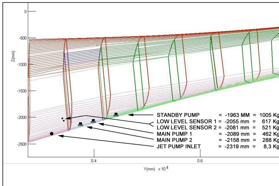
Figure 5. Inner fuel tank modeling (cross-section)
