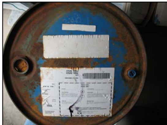
Photo 4. Second drum with weathered large bung plugs and no plastic seal. On delivery of barrel, the small bung plug did have a plastic seal.
