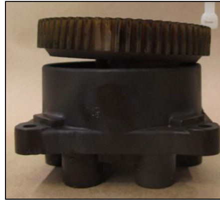
Photo 2. Displaced distributor rotor
