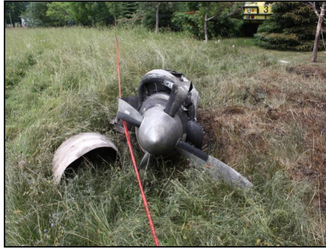
Photo 2. Damage to the right propeller
