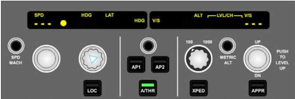
Figure 3. Flight control unit, showing the altitude selector knob (second from right), and the vertical speed/flight path angle selector knob (far right) (Source: Federal Aviation Administration, Accident Overview, Indian Airlines Flight 605, Airbus A320-231, VT-EPN)
