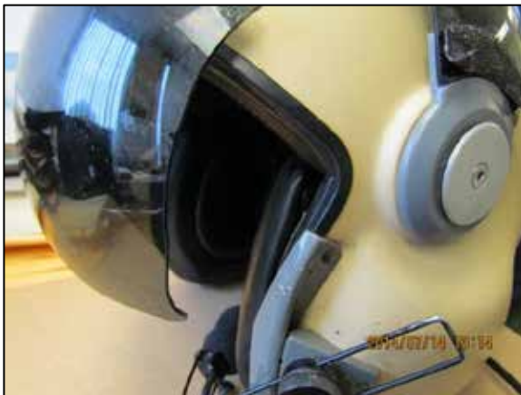
Photo 3. Pilot's helmet impact damage to left side visor (Source: Héli-Boréal)
