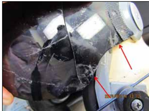
Photo 4. Pilot's helmet close-up view of the left side visor with impact damage (Source: Héli-Boréal)
