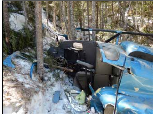
Photo 2. C-FHPC cabin floor (Source: Héli-Boréal)
