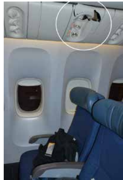
Photo 1. Passenger service unit damage at seat 35K
