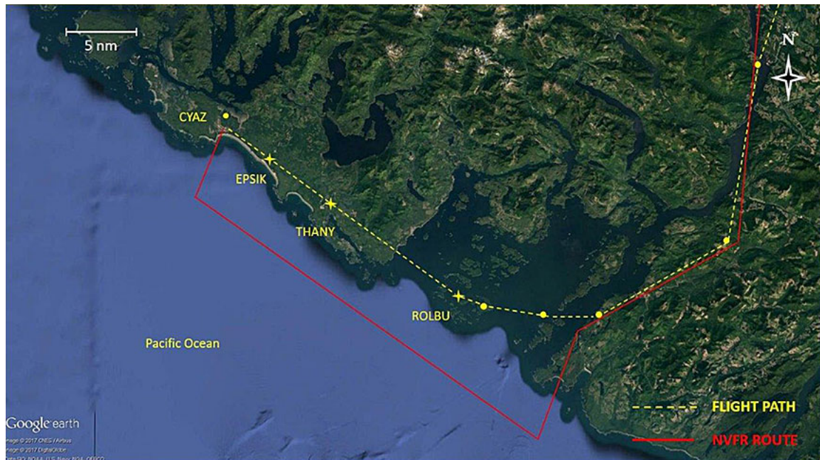
Figure 2. Night visual flight rules route and the helicopter's flight path (Source: Google Earth, with TSB annotations)
