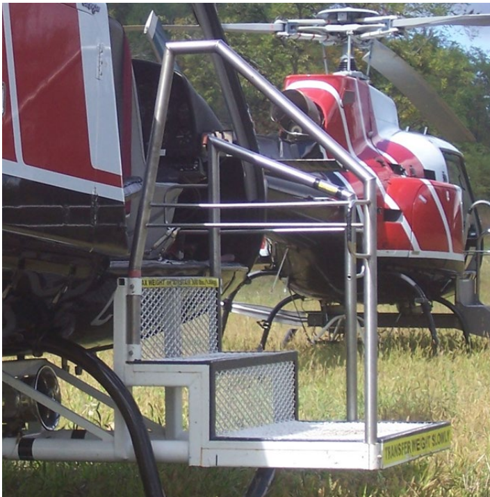
Figure 3. Helicopter with Air Stair attached (Source: Hydro One Networks Inc.)
