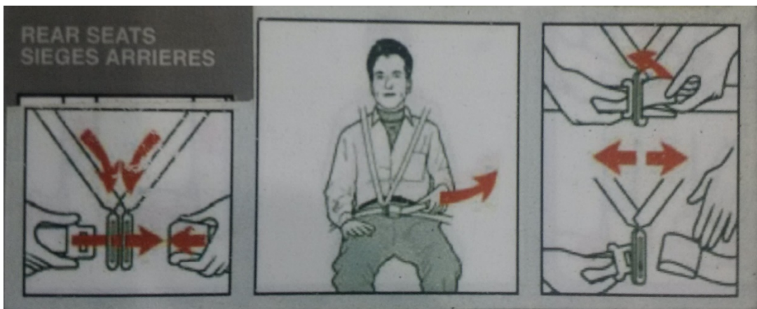
Figure 9. Hydro One's safety briefing card showing how to use the safety belts for the rear seats of the helicopter (Source: Hydro One Networks Inc.)
