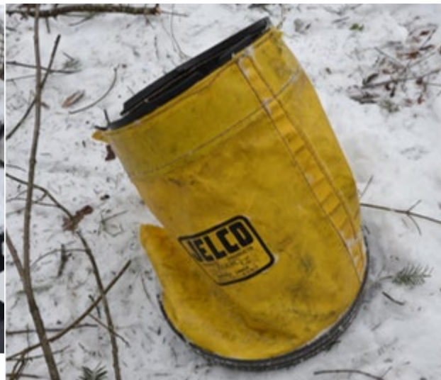
Figure 8. Nose bag that had become detached from the Air Stair and was found among the debris (Source: TSB)
