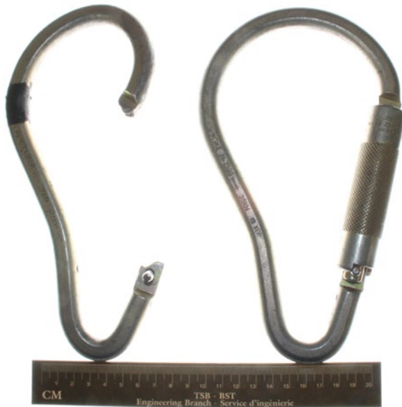
Figure 6. View of the accident carabiner (left) and an exemplar unit (right) (Source: TSB)
