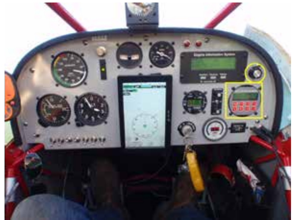
Figure 4. The occurrence aircraft's instrument panel showing the Simple Digital System programmer (yellow square outline) and mixture control knob (yellow circle outline) on the right of the panel (Source: Previous owner of the aircraft)
