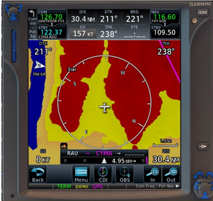
Figure 1. GTN 750 simulator display of terrain depiction based on GPS data entering Granite Creek at 4000 feet ASL. Magenta line is direct track between Rau Strip and CYMA (Source: Garmin, with TSB annotations)
