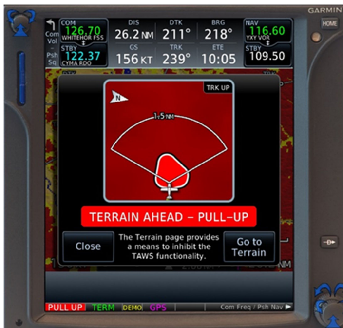
Figure 2. GTN 750 simulator display of terrain warning based on GPS data about 90 seconds before impact at 4000 feet ASL (Source: Garmin, with TSB annotations)
