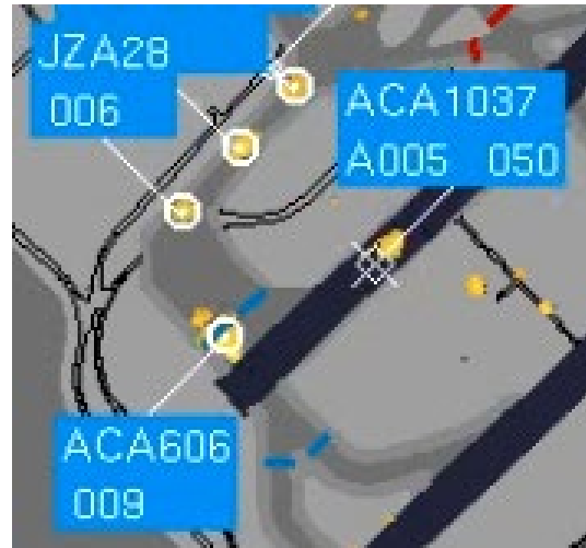
Figure 3. Screen shot magnification, taken at 0948:30, showing the change in status of the Embraer 190 (ACA1037) to in air at an altitude of 500 feet ASL (A005) and travelling at 50 knots (050) and the Boeing 777 (ACA606) travelling at 9 knots (009) (Source: NAV CANADA)
