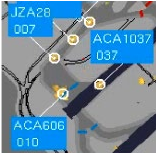
Figure 2. Screen shot magnification, taken at 0948:27, showing the track labels of a de Havilland DHC-8 (JZA28) travelling at 7 knots (007), the Boeing 777 (ACA606) travelling at 10 knots (010), and the Embraer 190 (ACA1037) travelling at 37 knots (037) (Source: NAV CANADA)
