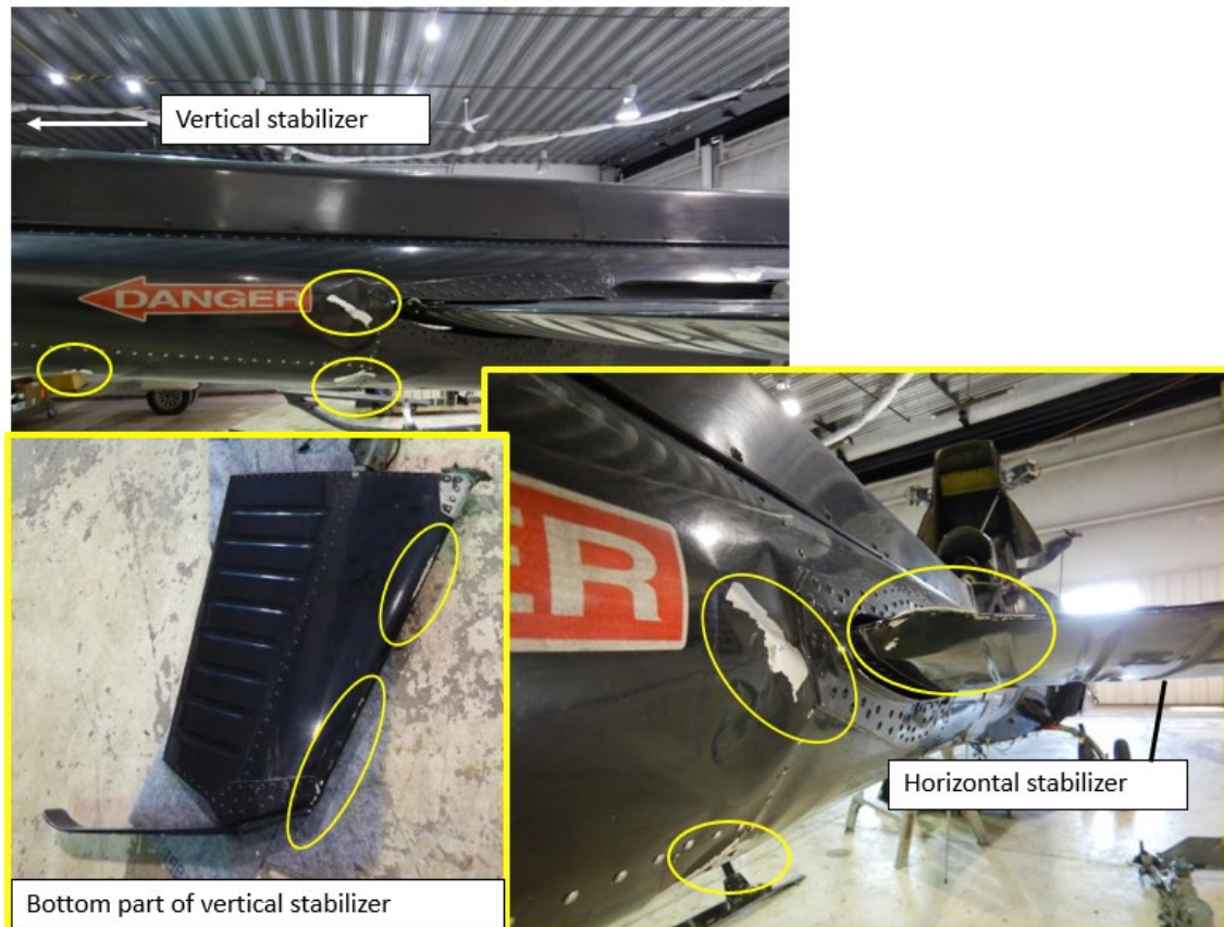
Figure 4. Photos showing the damage to the tail boom and horizontal and vertical stabilizers (Source: TSB)
