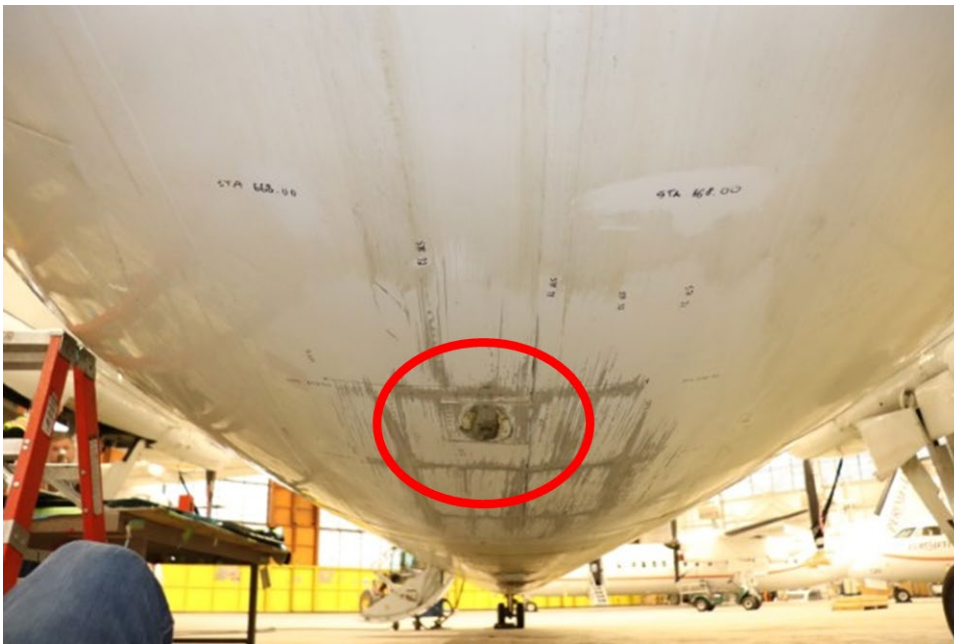
Figure 3. Exterior view of the occurrence aircraft's rear fuselage, showing the missing tail strike switch (Source: TSB)
