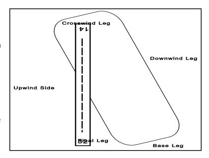
Canadian Aviation Regulations require that all turns be to the left while operating in the circuit, unless a right-hand circuit has been specified in the Canada Flight Supplement (CFS). The CFS specifies right-hand circuits for runway 32 at 108 Mile Airport during daylight hours.
