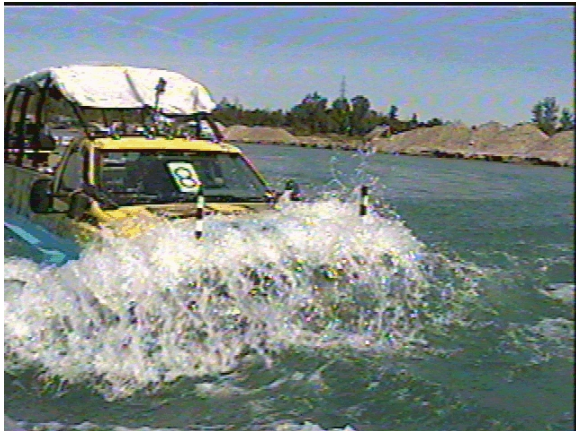
Photo 7. Vehicle speed of 8.3 km/h in disturbed water
