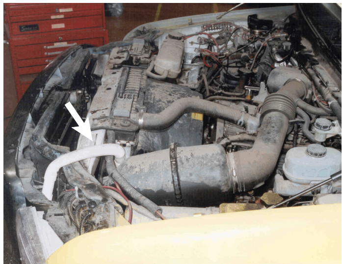
Photo 3. Discharge hose from the forward engine compartment
