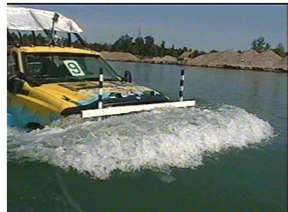
Photo 6. Vehicle speed of approximately 10 km/h in calm water
