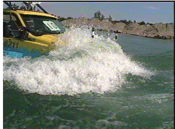
Photo 8. Vehicle speed of 9.75 km/h in disturbed water
