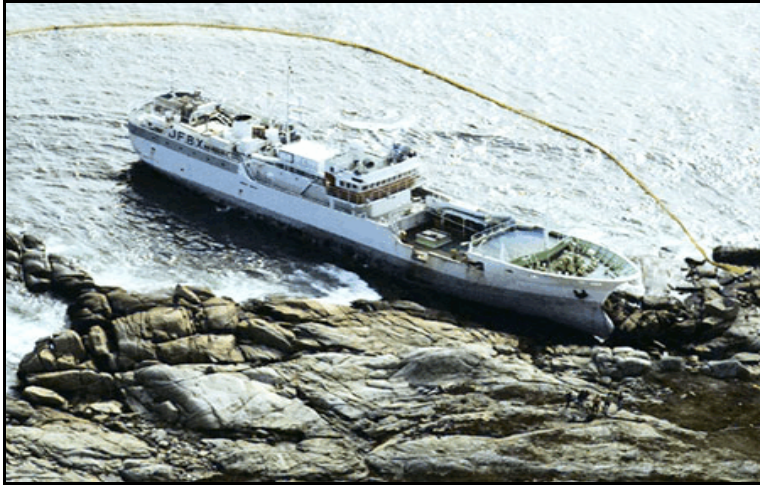
The grounded Shinei Maru No. 85 and oil spill containment boom
