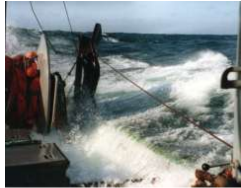
Photo 4. A wave breaks over the bulwarks and fills the deck, showing the importance of watertight integrity of vessels
