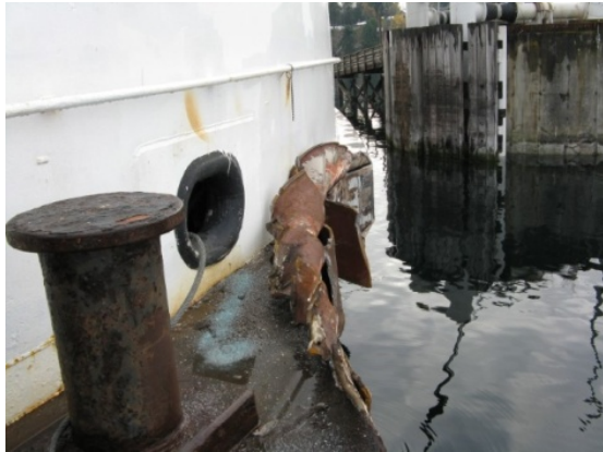
Photo 2. Damage to port rubbing strake
