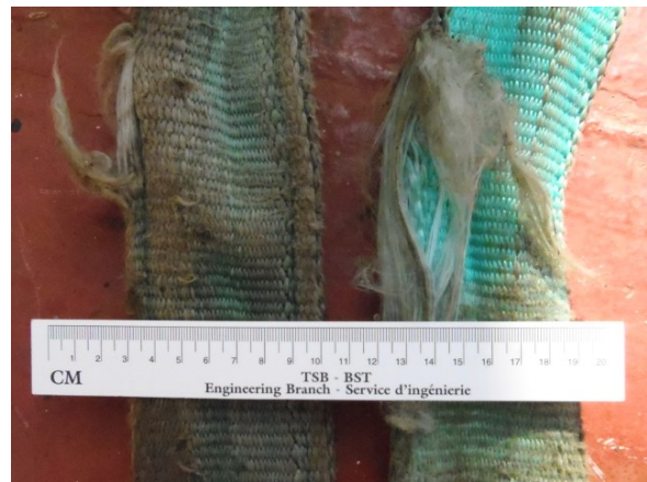
Photo 4. Extent of wear on the nylon slings
