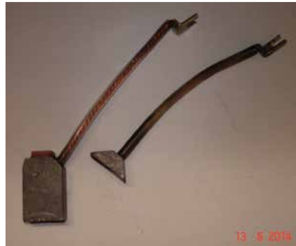
Photo 4. Comparison of a new brush (left) and the worn brush from the No. 1 generator (right)
