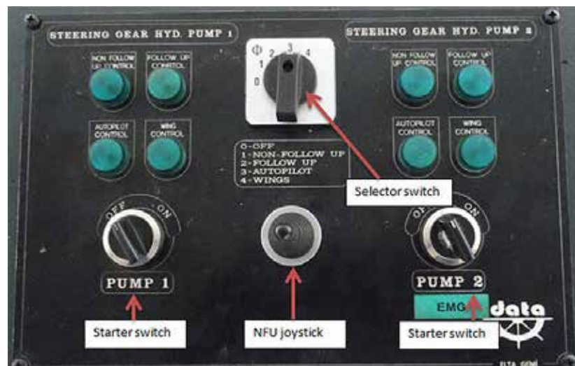
Photo 3. Close-up view of centre control panel
