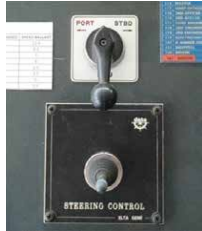
Photo 5. Wing console steering controls
